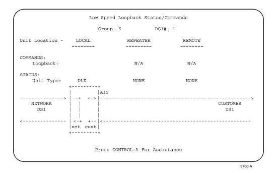
Figure 541-11b. DLX Network Loopback Screen
